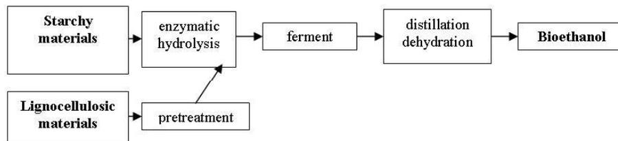
**Figure 1. The technology of obtaining ethanol**
